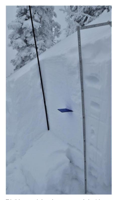
This 4' deep snowpit shows the new snow over the last 4 days: everything above the blue card, over 2' of snow measuring 2" of SWE. Avalanches are breaking on the very weak, sugary snow (facets and depth hoar) 1-1.5 feet above the ground. The smooth surface in the bottom left of the photo is the failure plane. Photo: GNFAC
