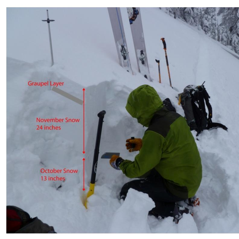
Just over 3 ft of settled snow as of November 16th can be found in the Bridger Range immediately north of Bridger Bowl. The main layer of concern is a combination of graupel crystals and heavily rimed, new snow crystals. A slightly denser layer of snow rests on top. These two layers are easy to find and will easily produce an avalanche if loaded by wind blown snow.
