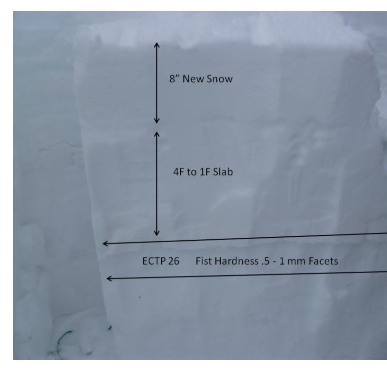
A layer of small grained facets buried 2 feet deep were propagating during stability tests. We found this layer in two different pits, E and NE aspects, and it produced unstable results in both locations. It took hard force to get this layer to fail, but the fact it was consistently propagating makes it untrustworthy. Photo GNFAC
