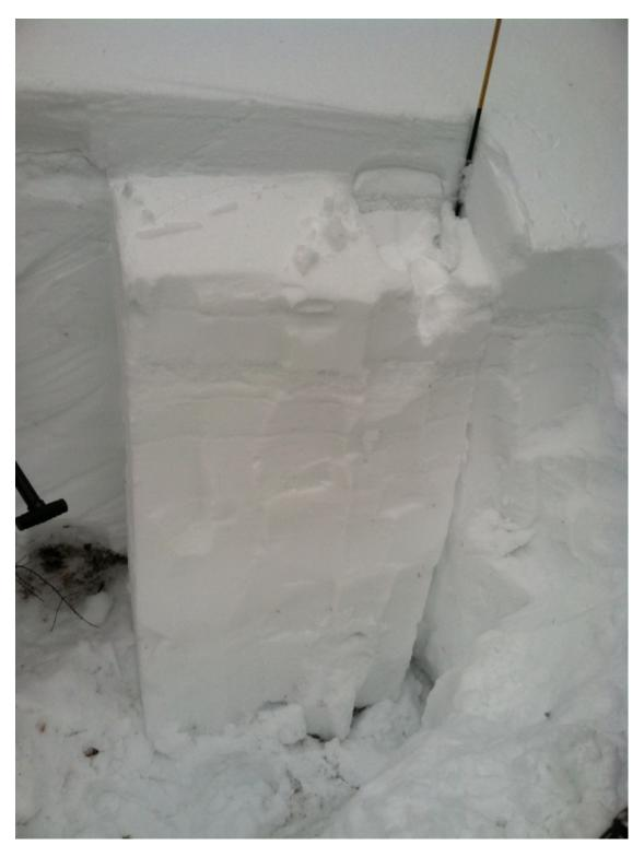
"Sun 3/16 we dug to the ground on a north aspect at ~ 8000 ft east of Emigrant peak and found 160cm of hard slab atop 20cm of very weak depth hoar. Though probably too deep for meaningful test results, this layer collapsed completely when isolating a CT column and on 10 taps in an ECT." Photo: J. Martin
