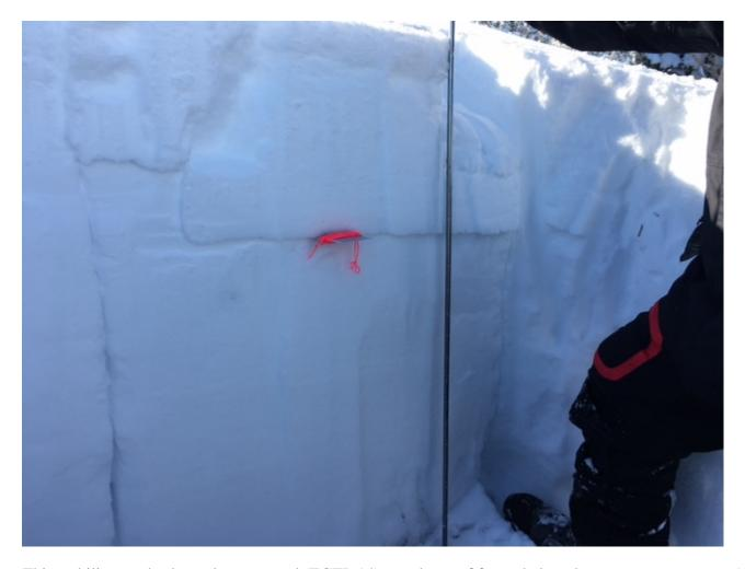
This stability test broke and propagated (ECTP 14) on a layer of facets below the recent storm snow. Avalanches are possible to trigger on this layer. Photo: J. Norlander
